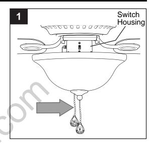
2. The pull chain located in the center is used to turn the *light* ON or OFF.
