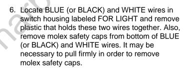
Connect WHITE wire from switch housing to WHITE wire from light kit fitter (D). Connect BLUE (or BLACK) wire from switch housing to BLACK wire from light kit fitter (D). Make sure that molex connections are secure.
