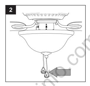
3. Use the fan reverse switch, located on the switch housing, to optimize the fan for seasonal performance. A ceiling fan will allow you to raise your thermostat setting in summer and lower your thermostat setting in winter without feeling a difference in your comfort.
