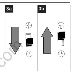
3c. **IMPORTANT**: Reverse switch must be set either *completely* UP or *completely* DOWN for fan to function. If the reverse switch is set in the middle position, fan will not operate.
