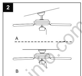
3. Check to make sure blades (F) are at least 30 in. from any obstruction. Check downrod (A) length to ensure blades (F) are at least 7 ft. above the floor.
