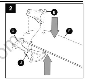
3. Place the plastic locking mechanism (E) on the opposite side of the blade (F) as the blade arm (G), refer to Fig. 2, with the *narrower* end of the plastic locking mechanism (E) toward the end of the blade (F) and against the blade screw (J) as shown in Fig. 3. [Please note the side of the plastic locking mechanism (E) indicating THIS SIDE UP.] Rotate plastic locking mechanism (E) to the left (counterclockwise) to lock plastic locking mechanism (E) into place.
