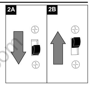
2C. **IMPORTANT**: Reverse switch must be set either *completely UP* or *completely DOWN* for fan to function. If the reverse switch is set in the *middle* position (Fig. 2C), fan will not operate.
