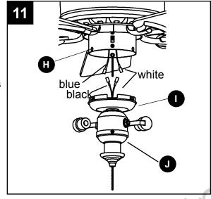
12. Attach the switch housing cover (I) to the switch housing (H). Align holes in switch housing cover (I) with holes on outer edge of the switch housing (H) (Note: The wide gap in the edge of the switch housing cover (I) should align with reverse switch on the switch housing (H).) Re-insert screws and secure all screws.
