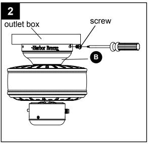
3. Directly align the locking slots of the canopy (B) with the two screws in the mounting bracket (A). Push up to engage the slots and turn clockwise to lock in place. Immediately tighten the two screws firmly. Install the two screws that were removed in previous step and tighten securely.
