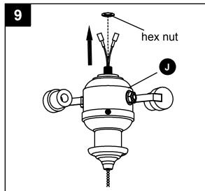
10. Insert the black and white wires from the light kit (J) through the center hole in the switch housing cover (I). Hold wires taut while installing switch housing cover (I) to prevent the wire from twisting. Tighten the light kit (J) onto the switch housing cover (I). Install the hex nut removed in Step 9.
