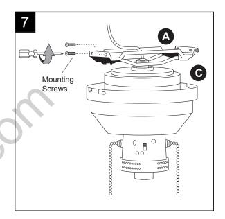
8. Attach the motor housing (C) to the mounting bracket (A) by aligning the two loosened screws into the two L-slots of the motor housing (C). Then turn the housing clockwise so the screws move toward the end of the L-slots. The housing should now sit securely on the screws preassembled on the mounting bracket (A).
